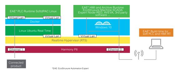
Windows can be updated and restarted on is own, without impact on the rest of the configuration. So, the soft PLC can independently manage the remote connected device without interruption. The automation engineer can remotely configure the different runtime software installed on either operating system, from his or her laptop with access to the necessary build time applications that run the project user files.
