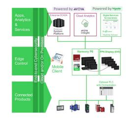
IIoT-enabled devices, gateways, edge boxes, and industrial PCs running at the edge of industrial automation control systems improve productivity and performance, becoming the next step in the digital transformation.
